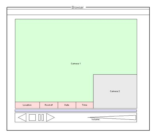
Video player shall display video from camera 1, a smaller inset of video from camera 2, location of the video, room number, date, and time. This information is required to identify video files. The PIP image should be adjustable in size during the initial system setup. In addition to PIP, therapist can select split image display with Camera 1 on the left side and Camera 2 on the right side. The final on screen layout will be determined during initial pilot system installation.
