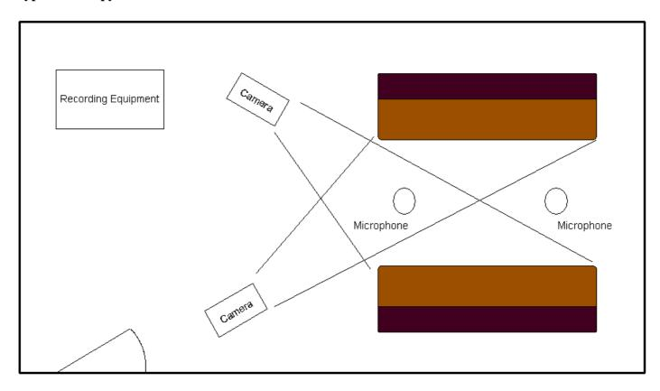
Typical therapy room contains two couches or chairs, two cameras, two microphones and the recording equipment. The recording equipment shall be located in a secure enclosure. Therapist shall have an easy access to recording control.
